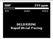
**Note:** The temporary pacemaker does not deliver RAP until the Enter key is pressed and held. **RATE**, **A OUTPUT**, **V OUTPUT** remain at their selected values for the current pacing mode until the Enter key is pressed and held.
