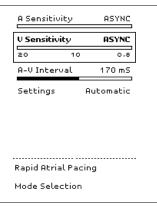
The pacing and sensing status bar indicators at the top of the upper screen reflect the change. The **SENSE** indicator under the **V SENSE** LED is not displayed, and the **V SENSE** LED no longer flashes.
