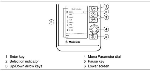
Figure 2. Controls and indicators for the lower screen
