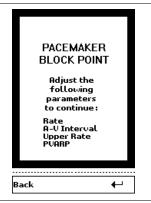
If the temporary pacemaker reaches a block point, press the Enter key and adjust one of the following pacing parameters:
