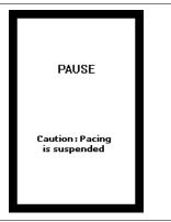
When the Pause key is released or pause times out at 10 s, the temporary pacemaker resumes pacing at the programmed parameters.
