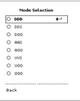
The Pacing Mode indicator in the upper screen displays the selected mode. The new mode is activated within the next two cardiac cycles.
