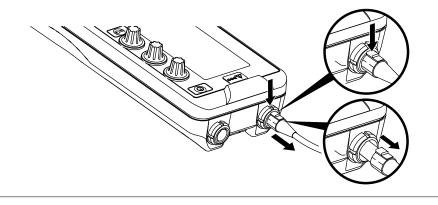
Figure 21. Disconnecting the cable from the temporary pacemaker
