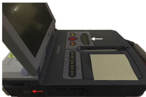
Fig 2. Zoom Latitude Programmer with the on/off switch and programming keys highlighted by a red and white arrow, respectively.
